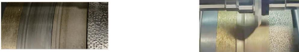
Note: the execution sequence is resin (PC), glass, edge polishing, flat polishing, edge fine grinding, flat fine grinding
