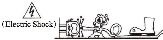
■ Avoid trampling or crushing of power cables. Do not pull or twist power cables; otherwise, fire and electric shock may occur
