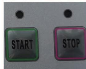
Start ■ Press the start button. Lens grinding begins (see Figure 8)
