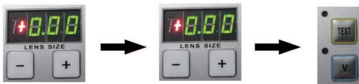
1 (FIG. 14) : Re-use "-"key to repair the size
