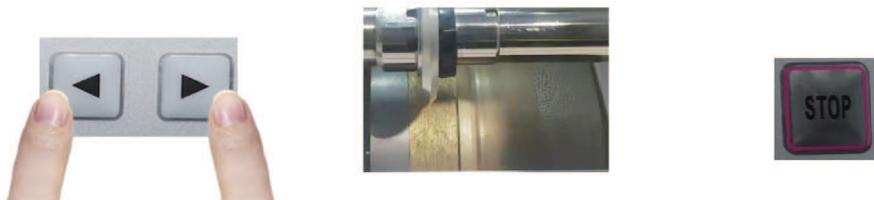
(5) When the standard template stops above the glass wheel, the < or > key can be used to make the template in the desired position, and then press the "Stop" key. After contacting the glass wheel, the standard template will move above the "V" groove grinding wheel.
