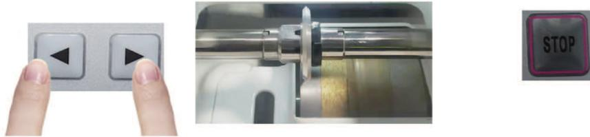
(4) When the standard template stops on the polishing wheel, the position can be moved by < or > key. Then press the "Stop" button, and after contacting the polishing wheel, the standard template will move to the top of the left glass wheel (see Figure 6).
