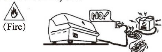
■ Do not use a power socket with other machines, power fluctuations can seriously interfere with the equipment and create a fire hazard.
